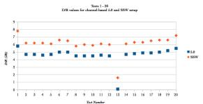
Figure 18: DRR results for all 20 measurements at mic position 1 for 5.0 setup (blue) and SSW setup (orange).
