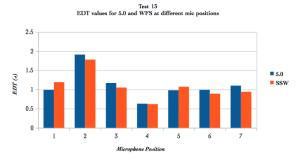
Figure 12: EDT values for test 13 from 5.0 setup (blue) and SSW setup (orange) at the 7 different mic positions.
