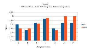
Figure 11: T30 values for test 4 from 5.0 setup (blue) and SSW setup (orange) at the 7 different mic positions.
