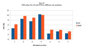
Figure 10: DDR values for test 4 from 5.0 setup (blue) and SSW setup (orange) at the 7 different mic positions.
