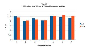
Figure 14: T30 values for test 13 from 5.0 setup (blue) and SSW setup (orange) at the 7 different mic positions.
