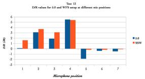
Figure 13: DRR values for test 13 from 5.0 setup (blue) and SSW setup (orange) at the 7 different mic positions.
