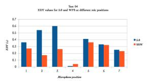
Figure 9: EDT values for test 4 from 5.0 setup (blue) and SSW setup (orange) at the 7 different mic positions.
