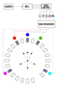
Figure 2: Loudspeaker array with chosen microphone positions for RIR measurements of the object-based SSW system. The virtual source positions are marked by colored circles.
